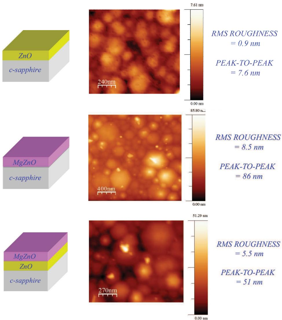
Figure 3. Tapping mode AFM images of the ZnO/sapphire, MgZnO/sapphire and MgZnO/ZnO/Sapphire surface morphologies.
