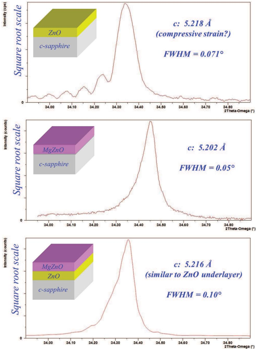
Figure 1. XRD 2 theta-omega scans of the (0002) peak for ZnO/sapphire, MgZnO/sapphire and MgZnO/ZnO/sapphire.
