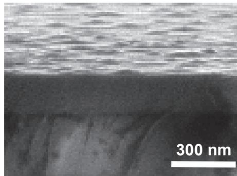
Figure 2. SEM image of a fracture cross-section of the MgZnO/sapphire sample.
