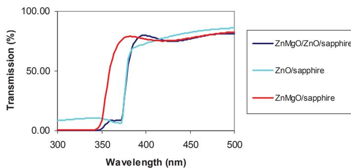
Figure 4. Optical transmission spectra for the ZnO, MgZnO/sapphire and MgZnO/ZnO/sapphire samples.
