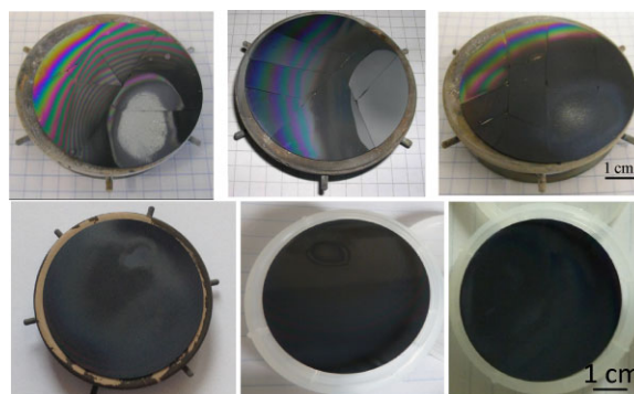
Figure 16 The three upper images show PLD-grown nanostructures on 2 inch diameter Si wafers without the use of optical rastering (N.B. wafers were deliberately cleaved before PLD in order to reduce the need to manipulate the sample after growth). The three lower images show PLD-grown nanostructures on 2 inch diameter Si wafers with optical scanning of the laser beam.
