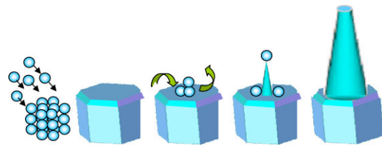
Figure 8 Illustration of a model for the formation of conical moth-eye nanostructures. The first stage represents the adatom arriving at the growth front. The third stage represents the renucleation of adatom which are not chemisorbed (after Wang et al. [27]).
